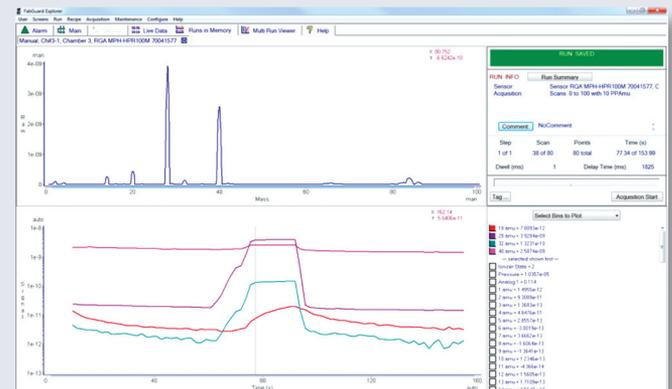
Air leak as can be seen by increasing signals of N<sub>2</sub> and O<sub>2</sub> in a 4:1 ratio
